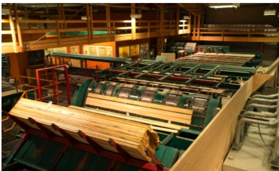
Figure 40 : Installation de triage (source : Blumer Lehmann AG)
